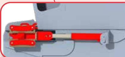
Hydraulic moving floor tensioner with automatic tensioning safety device.
